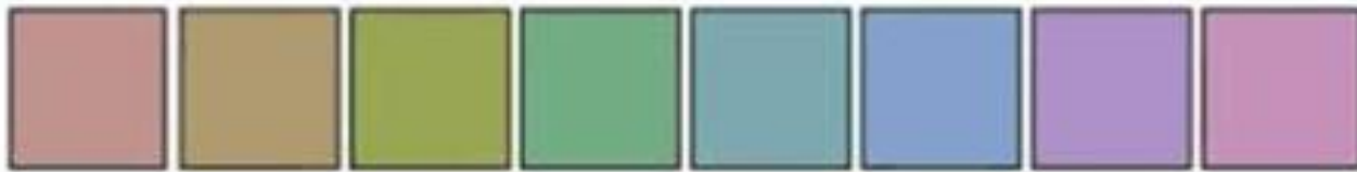
Figure 1. The eight color samples used in the calculation of Ra.
